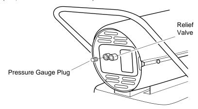
Figure 12 - Pressure Gauge Plug Removal
